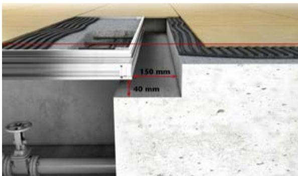
**Step 3:** A minimum rebate, 150mm wider than the over frame size and 40mm deeper (200mm for UniFace ASSIST and 160mm for UniTop ASSIST versions) than the over frame height of the access cover is to be provided for bedding and haunch material.
