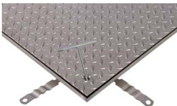
**Step 4:** For solid covers use at least two lifting/locking keys and insert the hook section of each key through diagonally opposite the locking positions (ASSIST versions in-sert keys into locking positions on the opposite side to the hinges). The cover is now ready to be opened/lifted.
