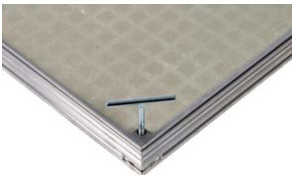
**Step 3:** For recessed covers use at least two lifting/locking keys and insert the threaded section of the key into diagonally opposite locking positions (ASSIST versions insert keys into locking positions on the opposite side to the hinges). Screw in both keys evenly until the cover raises slightly. Apply one more full turn to each key. The cover is now ready to be opened/lifted.
