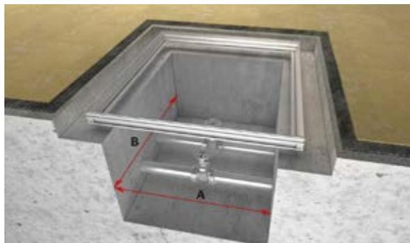
**Step 2:** Check that the shaft size is not larger than the clear opening dimension (AxB) of the access cover. The clear opening size of the access cover frame may be up to 20mm larger than the shaft size.
